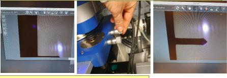
Adjust laser on the cantilever
