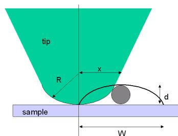
When imaging very small features, dull or blunt tips result in images with features that appear much wider than the actual size. With very sharp tips, the image width more closely represents the actual feature width. The height of the feature however, is accurately represented in both cases, for this idealized example. In a real imaging situation, sample compression and deformation also needs to be taken into consideration and can cause other imaging artifacts.
