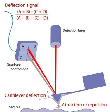
Most AFMs use a photodiode that is made of four quadrants, so that the laser spot position can be calculated in two directions. The vertical deflection (measuring the interaction force) can be calculated by comparing the amount of signal from the “top” and “bottom” halves of the detector. The lateral twisting of the cantilever can also be calculated by comparing the “left” and “right” halves of the detector.
