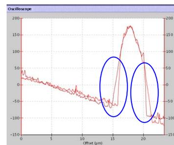
If the force applied to the surface is too high then structures will be displaced in the scan direction. This can also be detected in the oscilloscope. Usually the structures that start to move if the applied force is too high are flexible structures. The trace and retrace scan lines in the oscilloscope show these structures moving in the direction of the scan.
