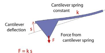
The four damping springs of a car's wheels have a higher spring constant than the spring in your ball pen. The spring constants of the commercially available cantilevers vary over four orders of magnitude; cantilevers with spring constants between 0.005 N/m and 40 N/m are commercially available. You can deduce the properties of a cantilever from its outer shape. Thicker and shorter ones tend to be stiffer and have higher resonant frequencies.
