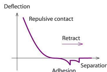
The force curves are often repeated at different locations to build up a map of the tip-surface interaction, or repeated many times at the same point to give a full statistical understanding of the interaction.
