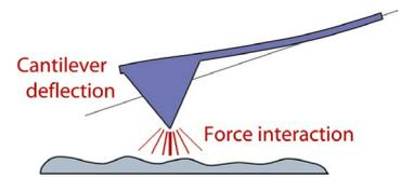
This cantilever deflection must be detected in some way and converted into an electrical signal to produce the images. The detection system that has become the standard method for AFM uses a laser beam that is reflected from the back of the cantilever onto a detector. The *optical lever* principle is used, which means that a small change in the bending angle of the cantilever is converted to a measurably large deflection in the position of the reflected spot.
