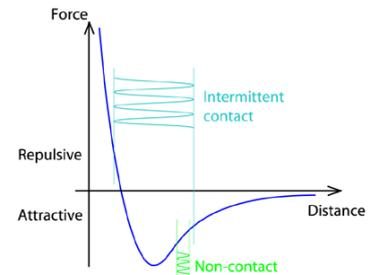
Non-contact mode is the only one that stays in the attractive part of the curve, but this makes it difficult to control, so it is not often used. In liquid, the attractive part of the curve may not be so obvious, and the oscillation is heavily damped, so it is not usually possible to use it on biological samples in liquid.
