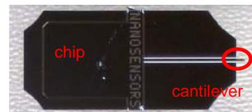
What you are unable to see without a good optical microscope is the tip at the end of the cantilever. Typically the tip is a few microns long, and shaped like a pyramid or a cone. The radius and angle of the end of the tip determines the imaging quality.
