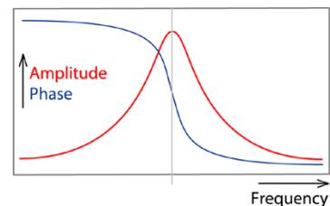
In intermittent contact mode, the setpoint value is the amplitude of the oscillation, so a higher setpoint value means less damping by the sample and hence a lower imaging forces.
