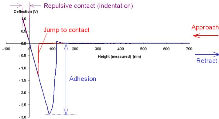
Typical interaction for an uncoated hydrophilic cantilever in air approaching a hard incompressible hydrophilic surface (e.g. glass or mica). Hydrophilic surfaces are covered with a thin water layer in ambient conditions. These layers join when the tip and sample are close together, forming a capillary neck between them and hence a strong adhesion.
