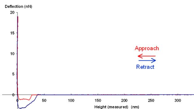
The example from above has had the x-axis corrected for the tip deflection. The x-axis is now the true tip-sample separation, rather than the piezo height measured directly.
