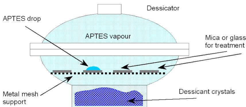
At the end, the droplet of APTES will have turned into a whitish silicate solid, this is not used, and the mica can be cleaved again to remove the reacted APTES. The other pieces of mica should now have reacted with the vapor. The surface is best
