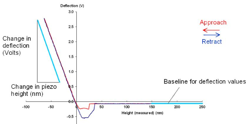
The gradient chosen for sensitivity measurements and the baseline offset for the deflection are both marked on this plot.
