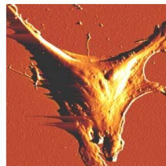
Error signal image of a fixed cell imaged at too high scan rate in contact mode
