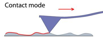
The lateral forces as the tip moves over the surface can be a problem in some situations, but can actually be an advantage in other situations. The lateral deflection can give information about the friction force between the tip and the sample, and can show up areas that may have the same height, but different chemical properties.
