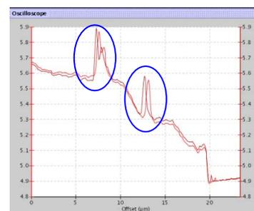
It can happen that the force applied to the cell is such that the tip starts to drift away from the surface at the edges (see arrows in image on the right) while still displacing a structures (blue circles). It may be that the structures in question are extremely flexible and will always be somewhat displaced. However, the user could try either a) increasing the gains, or if this leads to oscillations b) decreasing the scan speed and then decreasing the force.
