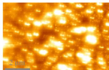
Another example of repeatedly occurring features caused by a dull tip. Here the tip is quite blunt, and has a triangular shape.
