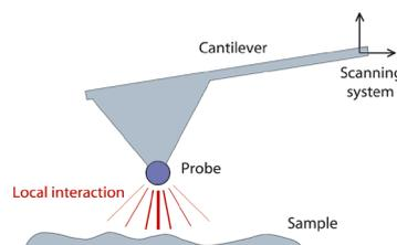
The idea of a probe measuring a local interaction and building up an image is relatively straightforward, but the actual implementation of a system with a resolution in this range is technically challenging. Many factors came together in the development of scanning probe microscopy, including the development of piezoelectric materials that made it possible to reproducibly position and scan components with a sub-nanometer precision.
