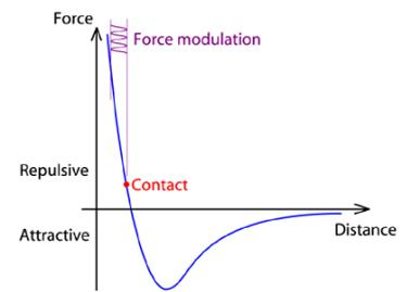
Intermittent contact mode moves between the attractive and repulsive parts of the curve. The maximum force perpendicular to the sample may be higher or lower than in contact mode, but this is only applied for a short part of the cantilever cycle. Therefore the sample damage and lateral drag can both be reduced compared with contact mode for some samples.
