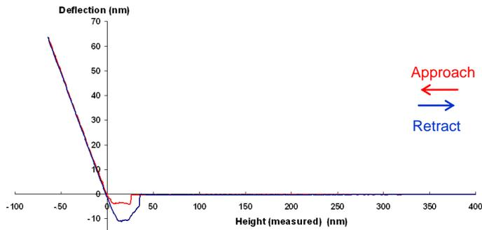
The sensitivity is the conversion factor (nm true deflection per Volt measured deflection) needed to convert the photodiode deflection into units of length.
