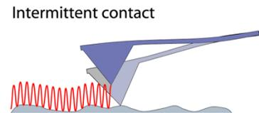
The cantilever is usually driven close to a resonance of the system, to give a reasonable amplitude for the oscillation and also to provide phase information. The phase of the cantilever oscillation can give information about the sample properties, such as stiffness and mechanical information or adhesion. The resonant frequency of the cantilever depends on its mass and spring constant; stiffer cantilevers have higher resonant frequencies.
