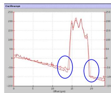
If the force is reduced too far the scan lines will differ more and more at the edges of the cell until the tip loses the surface entirely. When the oscilloscope looks as it does to the right it will be obvious in the scan that the tip is not properly tracking the surface (see error signal image below, black arrows).
