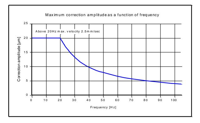
**Note:** At frequencies around 0.5Hz, even though there is no isolation at these frequencies, the system will be driven into saturation by amplitudes of around  $10\mu m$ . This will not normally be a problem unless you are working at the top of a very tall building.
