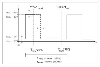
If no signal is present the pump accelerates up to its final rotation speed. A PWM adapter box for rotation speed setting operations for the turbopump is available as an option (please see Section 11. Accessories).
