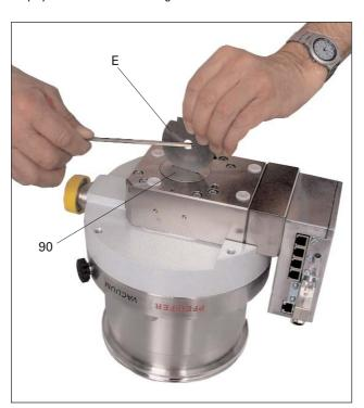
→ Use two screwdrivers to lift the lubricant reservoir 92.
