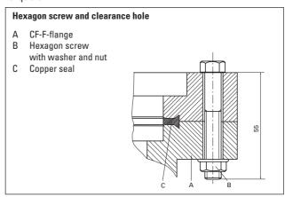
The components for installing to an CF-F flange are to be ordered under the following numbers:
