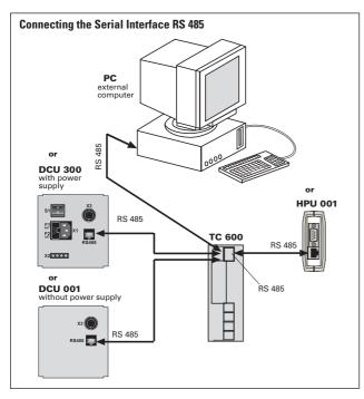
The serial interface is galvanically and safely separated from the maximum supply voltage from the TC 600.
