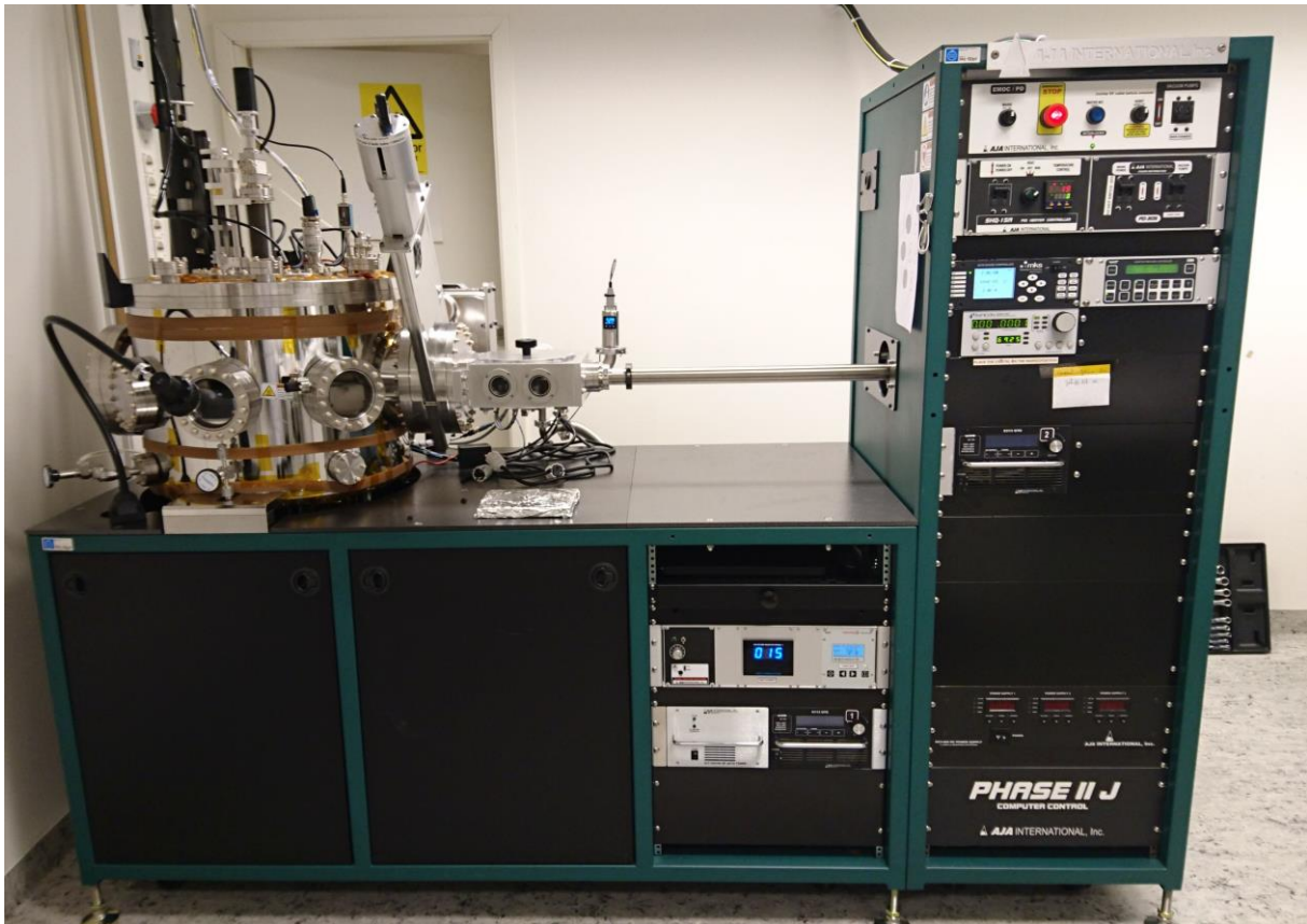
Overview of the system. To the left is the chamber, with the loadlock in the middle, and the electronics rack to the right.
