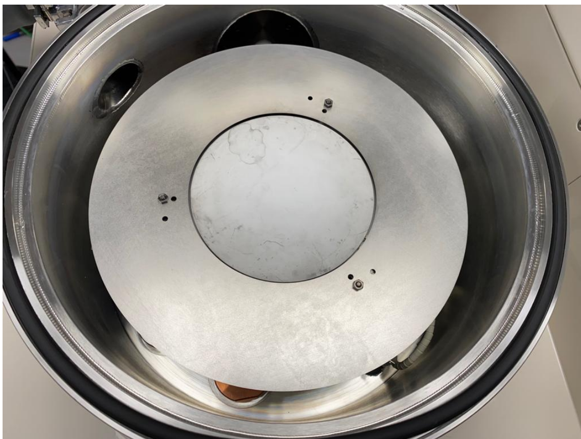
Figure 9: Photograph of a resistive element substrate heating stage inside an ANNEAL chamber.
