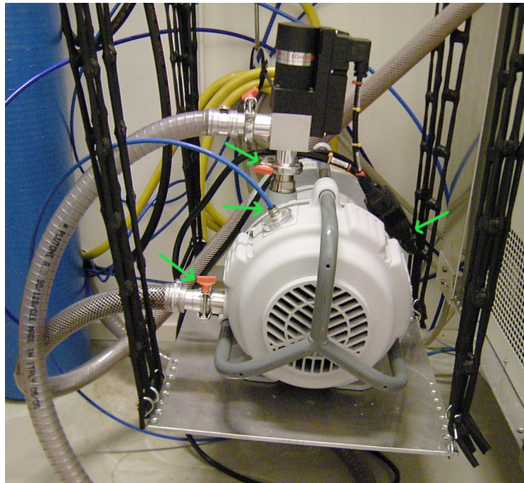
Backing pump on vibration free platform. Unmount inlet and outlet vacuum tubes, N 2 purge and mains voltage connector (green arrows).
