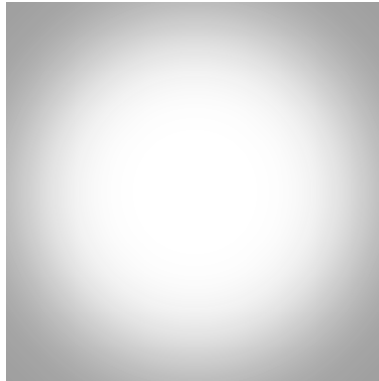
Figure 5.2. Example of a shading image showing inhomogeneous illumination
