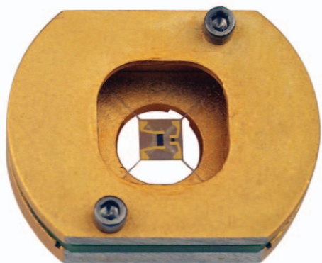
Dilution Refrigerator / Helium-3 2D Heat Capacity Puck
