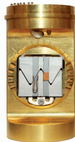
Dilatometer Capsule with copper sample
