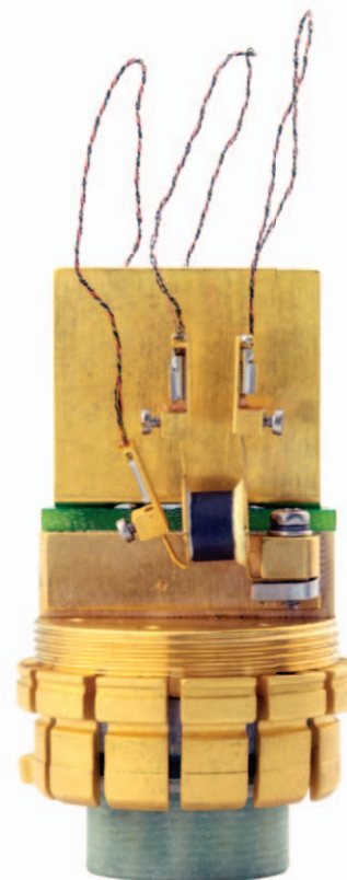
TTO Puck with Disk-Shaped Sample Installed
