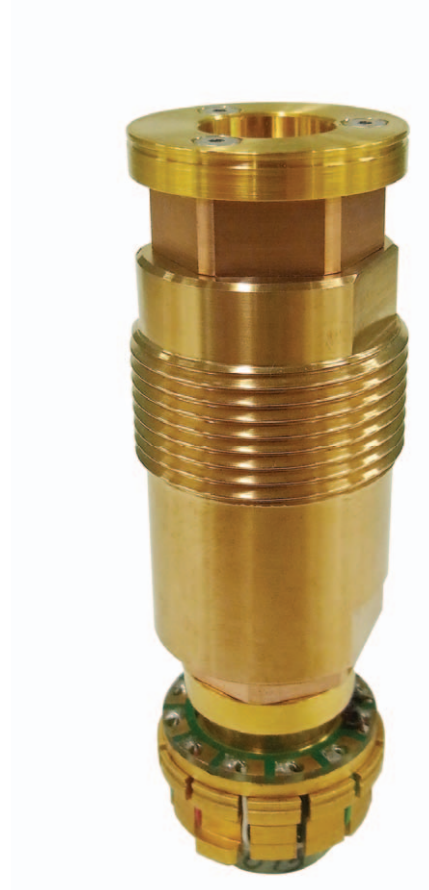
High Pressure Cell for Electric Transport Measurements
