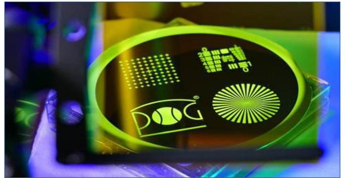
Fig. 21 Yellow fluorescent PMMA-based resist architectures
