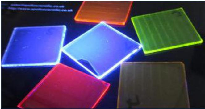
Fig. 19 Intensely fluorescing films of CSAR 62 on glass.
