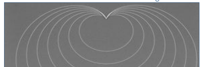
Fig. 3 Chrome structures with 20 nm lines after lift-off
