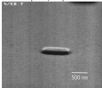
Fig.: 0.8 µm wide niobium dot after resist remove
