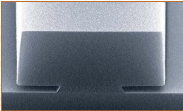
LOL 2000 on Si at 200 °C/ 5 min. with 5.0 micron SPR950
