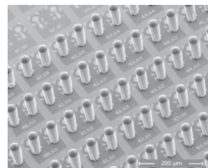
Replicated sol-gel refractive microlenses on a VCSEL wafer substrate (Courtesy of Avalon)
