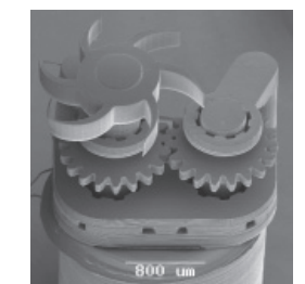
Windmill for fluidic media with a gearwheel connection produced with 3D-layer by layer UV-direct prototyping
