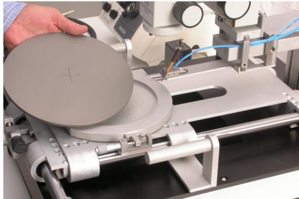
*Fig. 11: Inserting the chuck*
