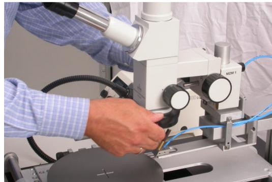
*Fig. 16: Adaption of the microscope and the ring light*
