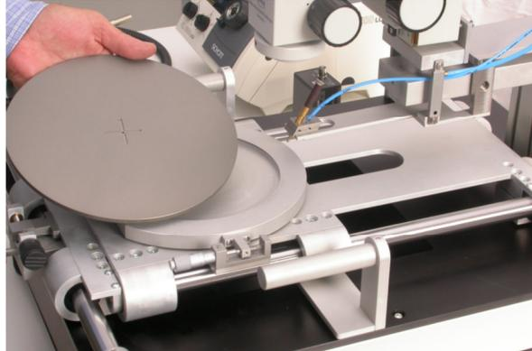
*Fig. 11: Inserting the chuck*
