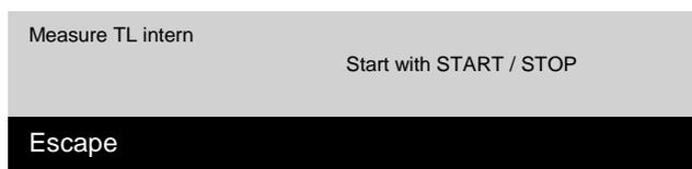
Actuating the **Start-key** Starts the measuring of the internal leak.
