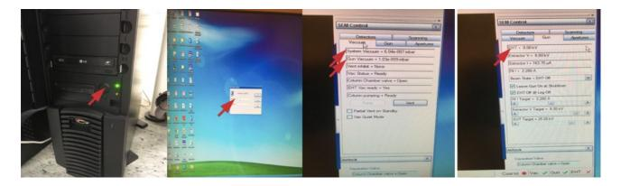
Log on to left computer, check vacuum of main chamber and gun chamber. If vacuum is ok  $(1x10^{-9} \text{ for gun chamber}, < 4-5 \times 10^{-6} \text{ for main chamber})$ , start the gun and the EHT. Run the Gun monitor logger for a couple of hours with EHT at 25 kV to check stability.
