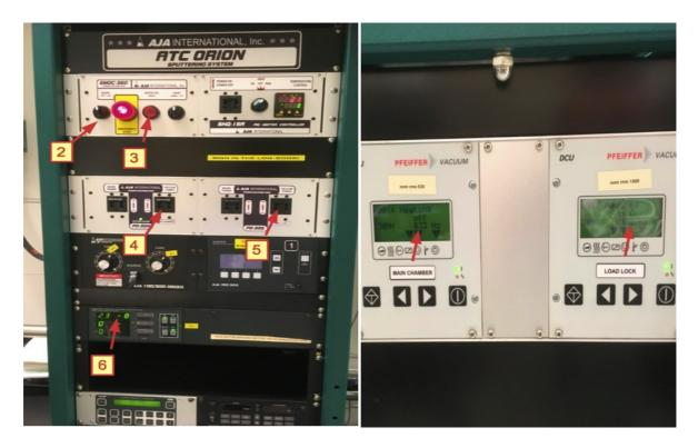
When the pump is at full speed the gauge controller pressure of the main chamber (6) starts to be active and we can see the pressure go down. After this you need to go in the software and start the bakeing of the chamber from the program. You can use the system after 12 h when the vacuum is in the range of the  $10^{-8}$  Torr.
