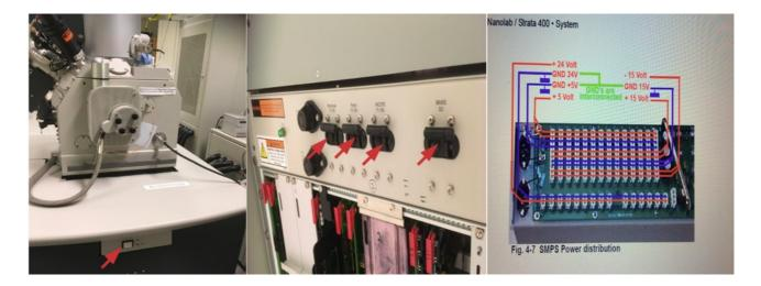
Normally the system can be started with the front panel button indicated in the picture to the left. One press and the button should be illuminated.
