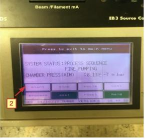
In order to start the system you need to press the Reset bottom (1) if is blue. Then you follow the screen controller START and PROCESS. After few minutes you may see the pressure into the system in range  $10^{-7}$  mBar.
